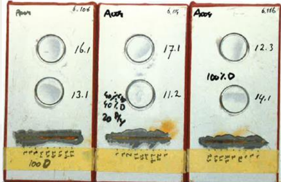
Photo 3: Seawater immersion test, panels 6.106, 6.114 and 6.116.
